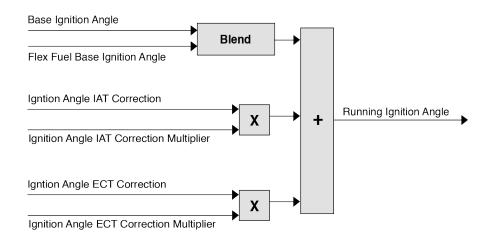
The final output of the module is derived by selecting the appropriate angle for the current engine state and then applying the maximum and minimum ignition angle limits.
