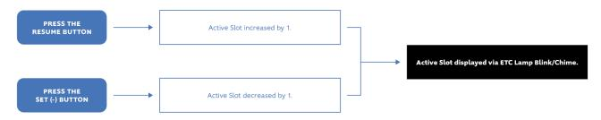
Active Slot will be limited to the Max Allowed Slots calibration setting.
